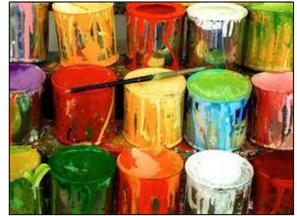
Unused latex paint should be opened to air dry before disposing into dumpster. Make sure paint is opened in a confined area and that there is no possibility that it could be spilled onto the ground or into or near the drainage system. It is illegal to dump or rinse paint into the stormwater system.
